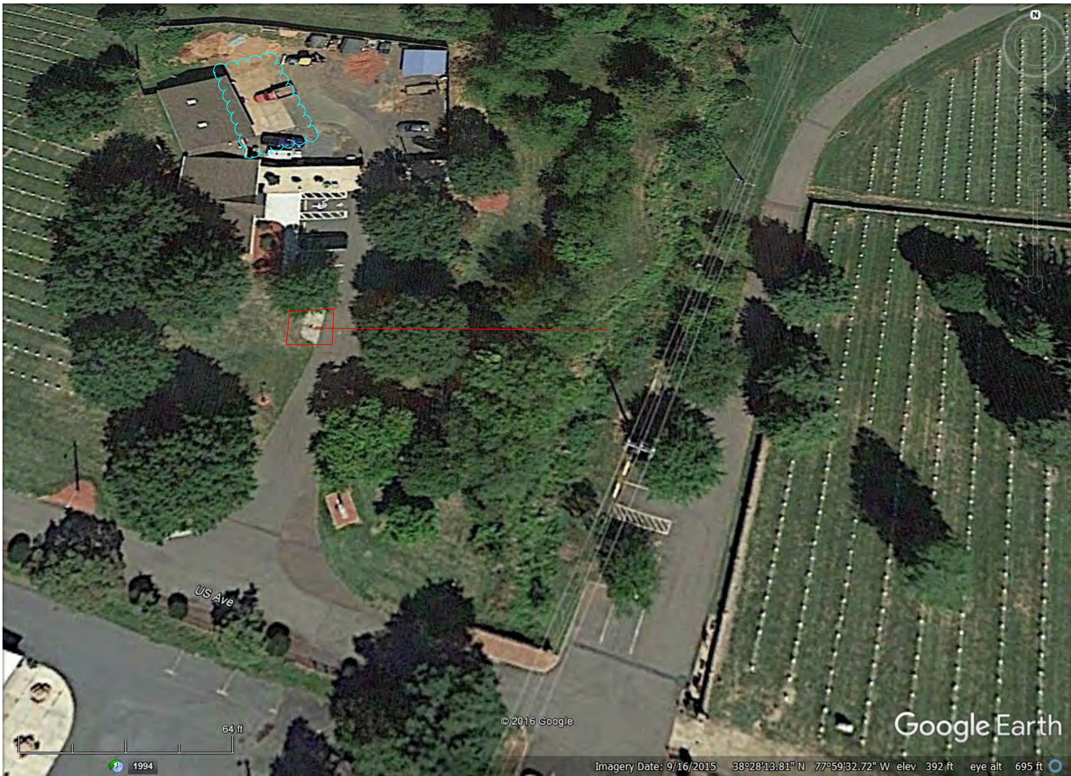
Detail 1: Site plan for work items near maintenance and administration buildings. The light blue bubbled area highlights the area for concrete replacement. The red square highlights the area for a replaced drain inlet. The red line highlights the route of underground drain piping to be piped to discharge into the river.
