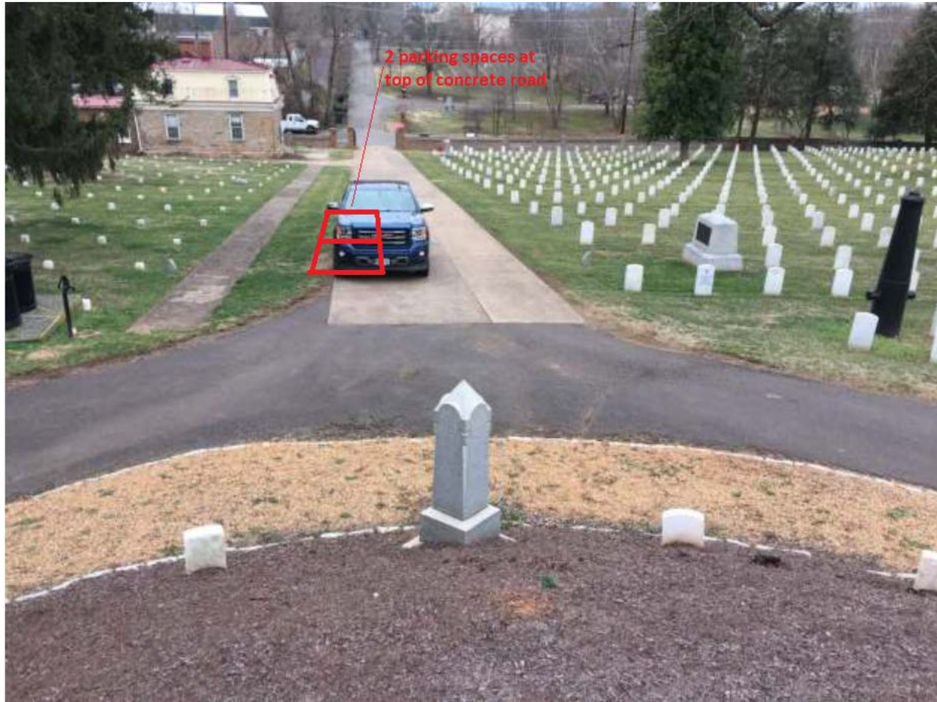
Detail 6: Add concrete as shown in red in the attached picture above to extend concrete roadway such that two parking spaces are created. Parking spaces shall be 9'x18' of which, as shown above, one-third is new concrete extension and two-thirds is utilizing the existing concrete roadway. Stripe parking spaces.
