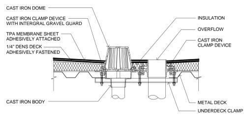
**15 ROOF DRAIN AND OVERFLOW**
