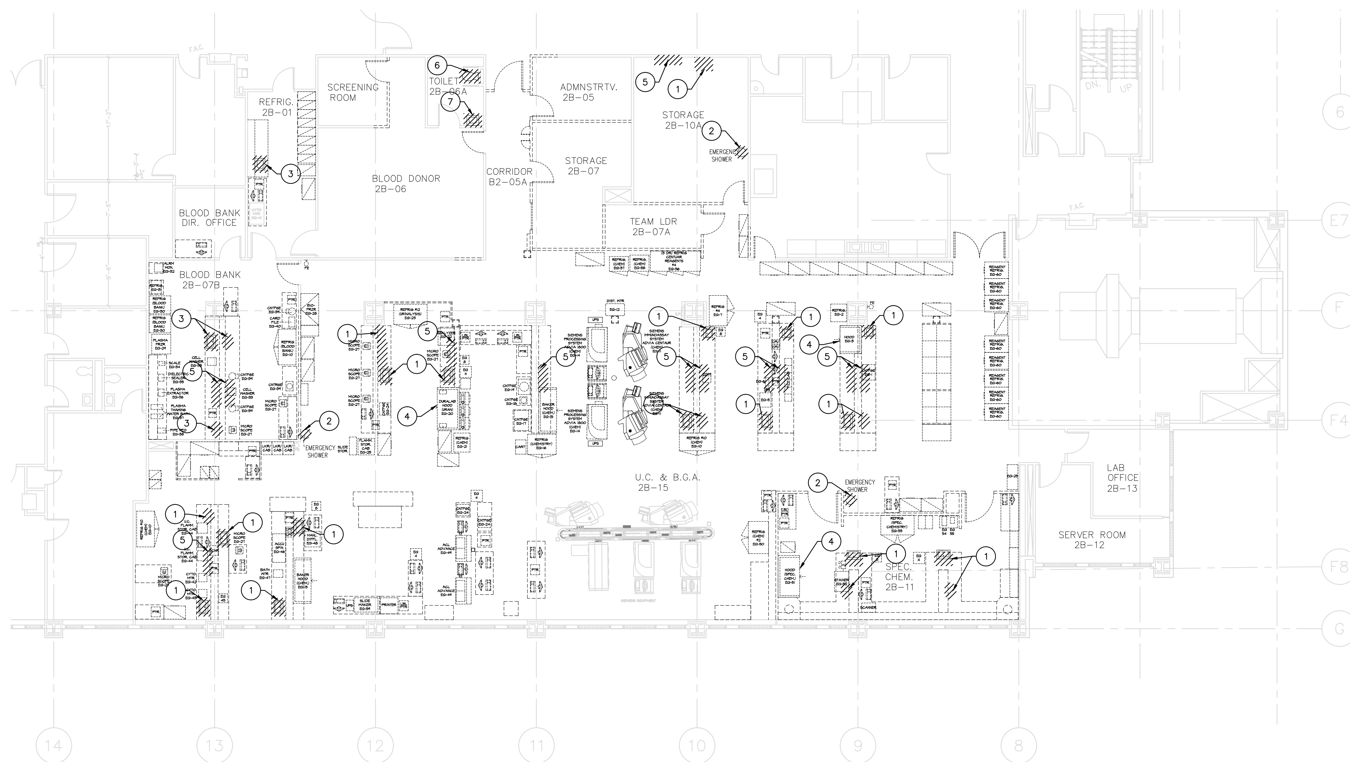
PLUMBING SECOND FLOOR DEMOLITION PLAN
