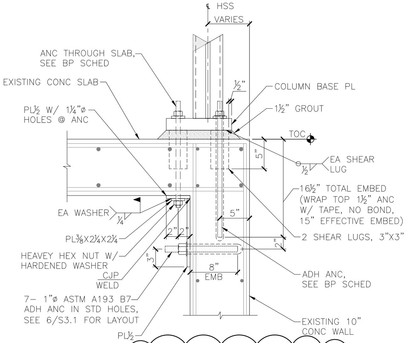
NOTE: LOCATE ALL REINF BEFORE INSTALLING ANCHORS. DO NOT CUT ANY REINF. NOTIFY ENGINEER OF CONFLICTS IN FIELD.
