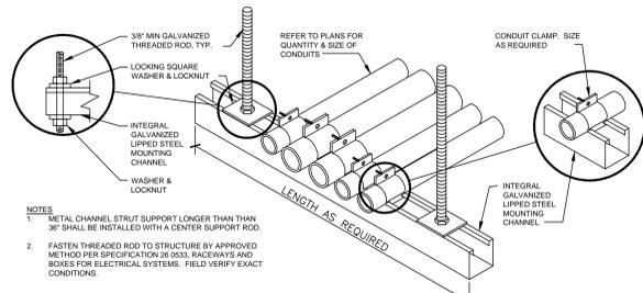
**E1 CONDUIT TRAPEZE MOUNTING DETAIL**
