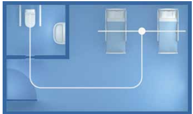
A linear track over the beds connects to a turntable and curved track section – to provide access for toileting.
