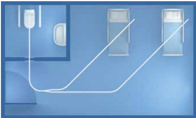
Two linear, angled tracks over the beds connect to an exchanger, which links to a curved track section for toilet access.
