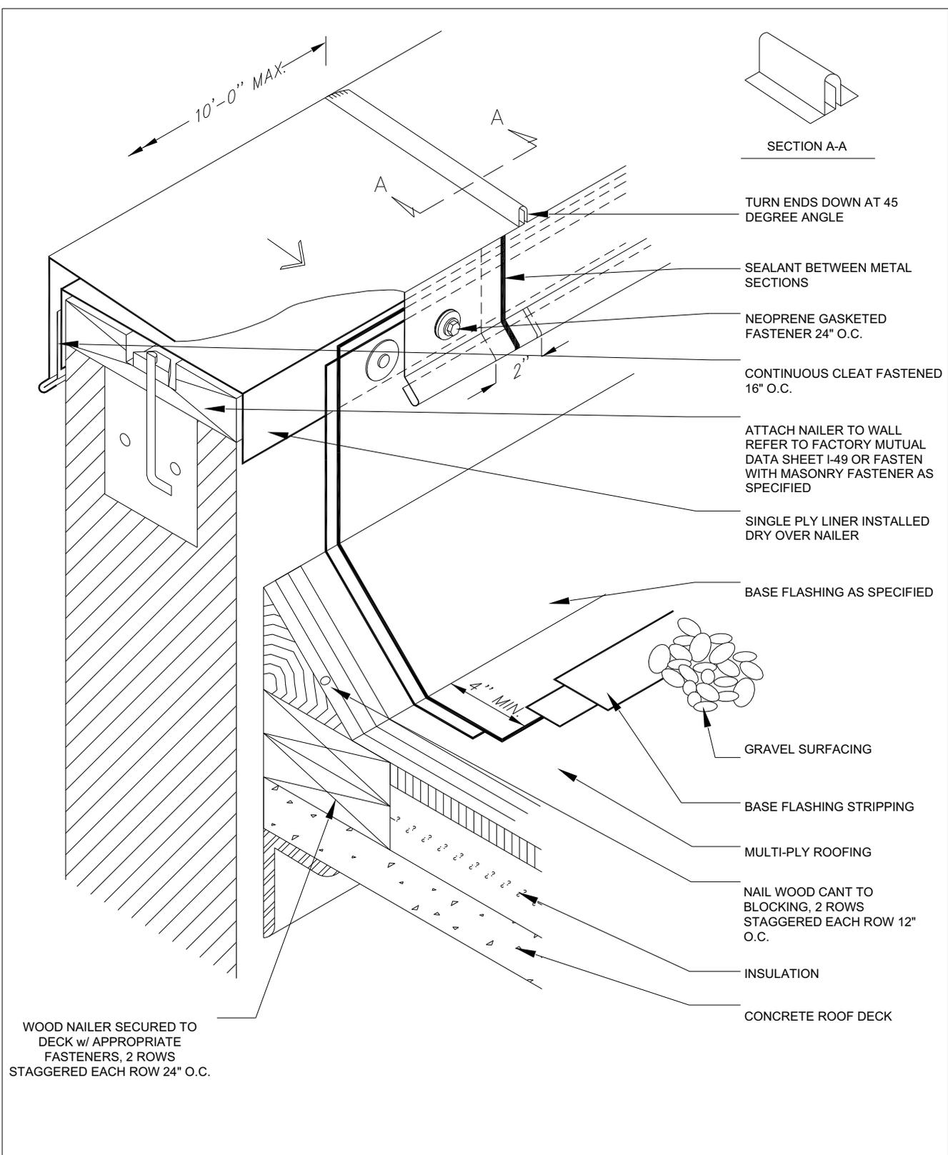
WOOD NAILER SECURED TO DECK w/ APPROPRIATE FASTENERS, 2 ROWS STAGGERED EACH ROW 24" O.C.
