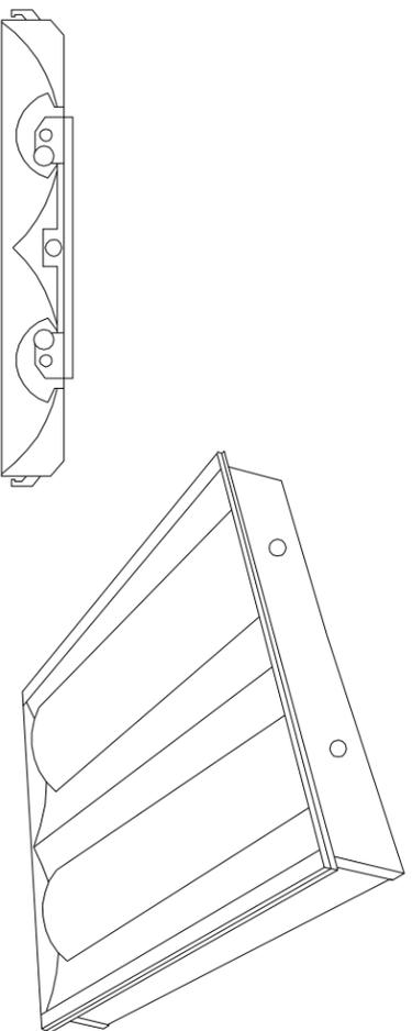
RECESSED, 2-LAMP, DIRECT-INDIRECT LUMINAIRE, FOR LAY-IN GRID MOUNTING WITH CLEAR PRISMATIC LENS PANEL. NOMINAL 2' X 4' IN SIZE AND APPROXIMATELY 3-5/4 INCHES DEEP.
