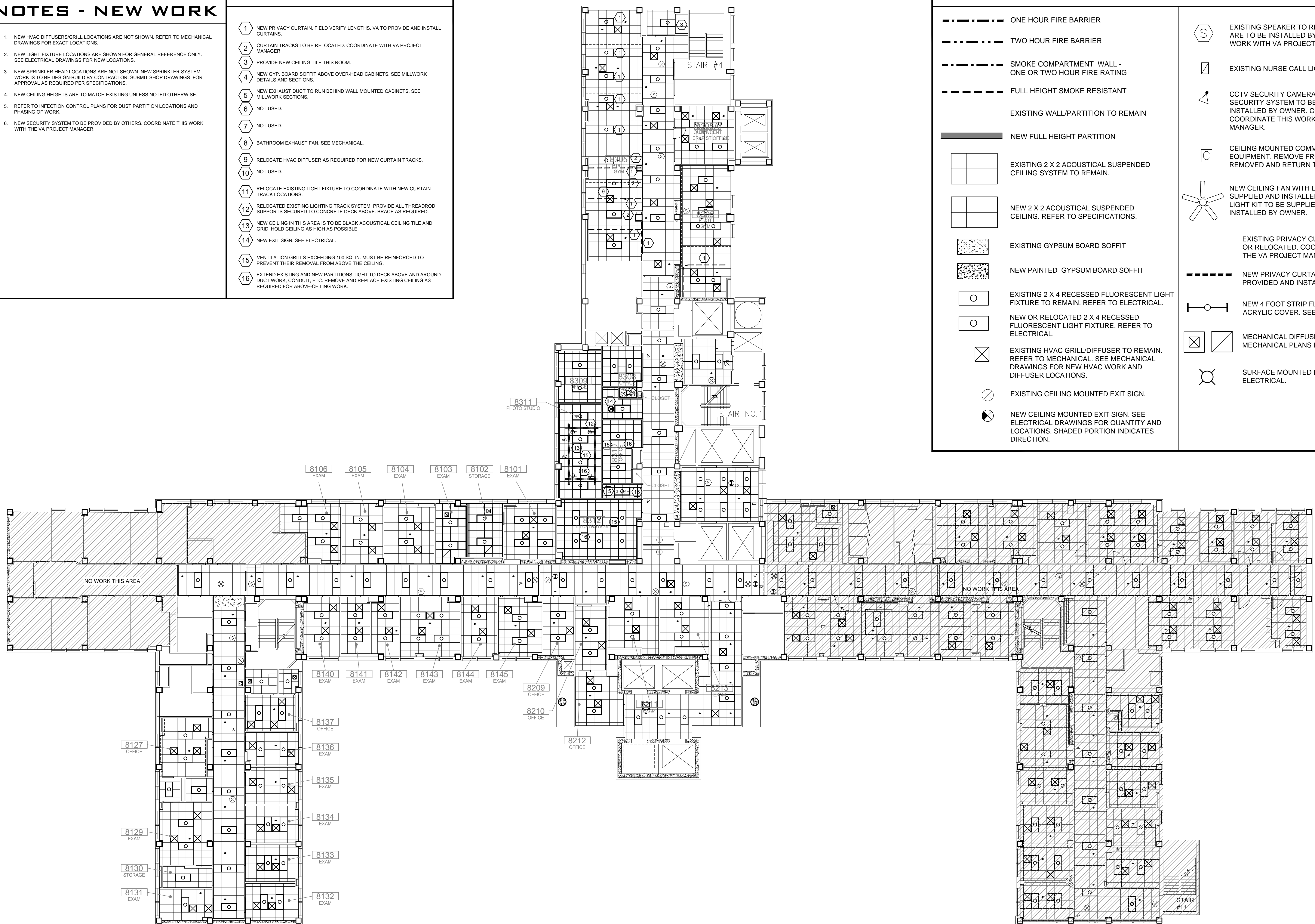
1 8TH FLOOR REFLECTED CEILING PLAN - NEW WORK SCALE: 3/32"= 1'-0"
