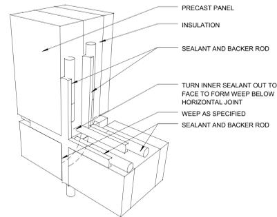
**E6 TYP TWO-STAGE SEALANT JOINT AT PC-1**
