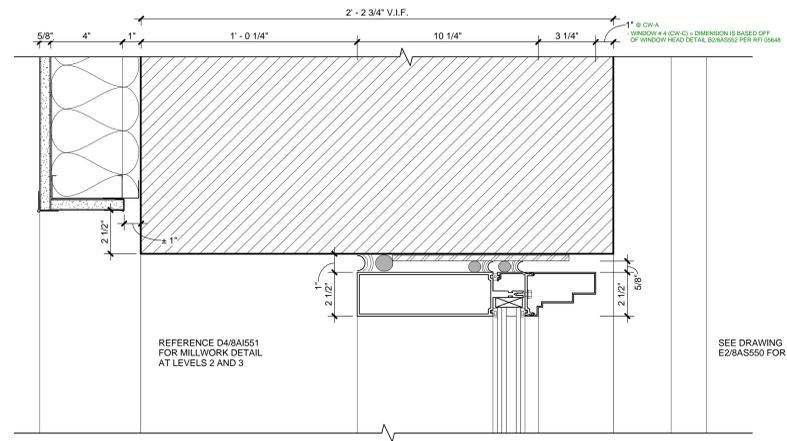
**D2** SECTION THRU DIXIE INFILL WINDOW JAMB AT LEVEL 1 TULANE MASONRY WALL
