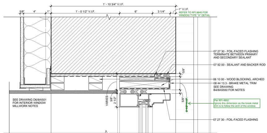
**F4** SECTION THRU DIXIE INFILL WINDOW AT ARCHED HEAD CONDITION
