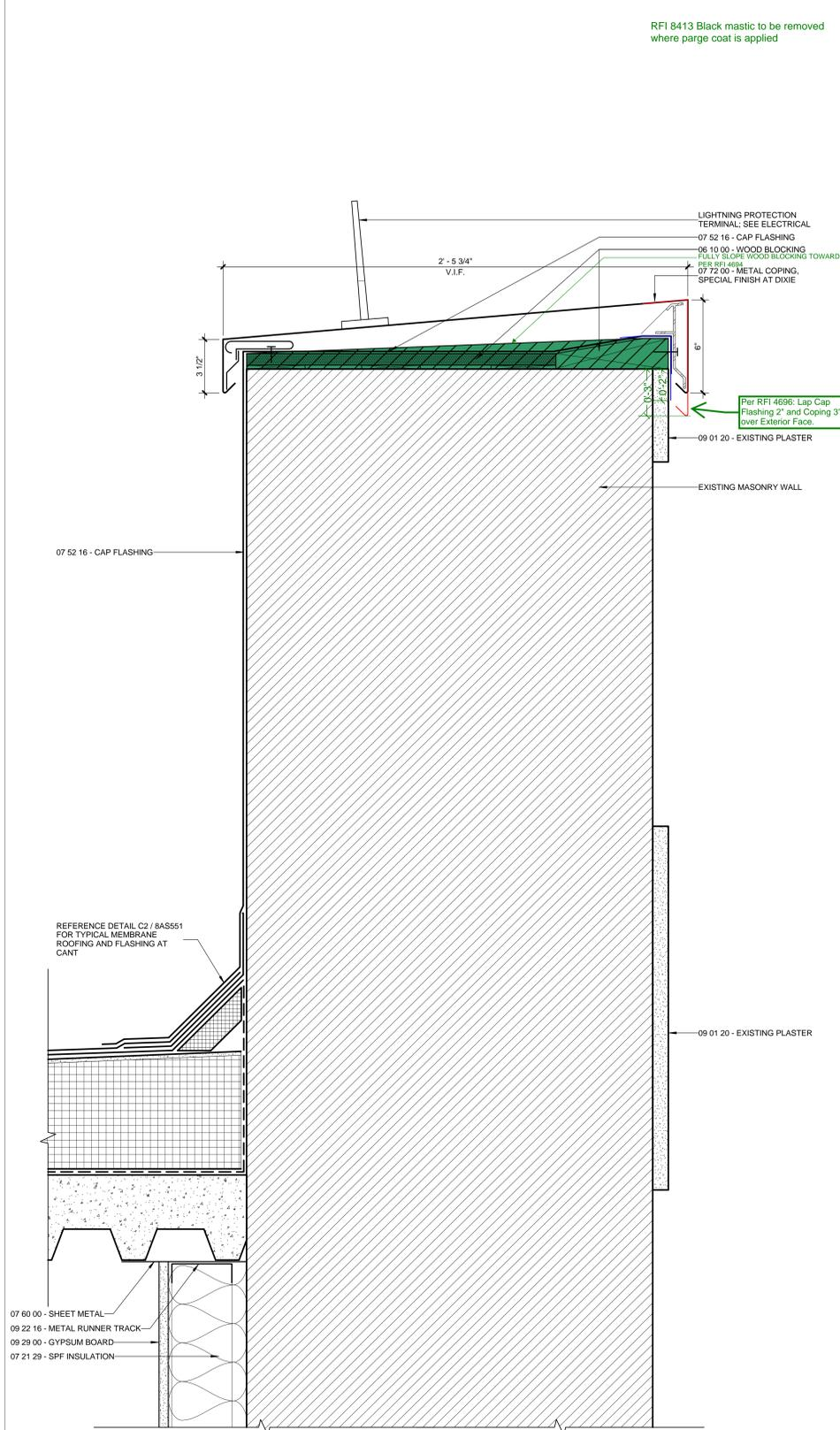
**F6** SECTION THRU DIXIE TULANE WALL AT MASONRY PARAPET
