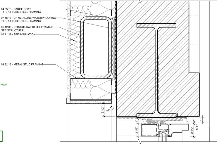
**B4** SECTION THRU MASONRY WALL AT TUBE STEEL STRUCTURE (TYP.) INCLUDING BLAST PROOFING STEEL RFI 06643
