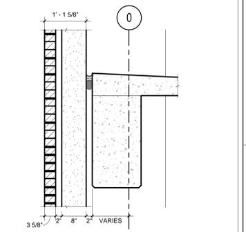
TYPICAL CAST-IN-PLACE TO PRECAST/FACE BRICK SECTION
