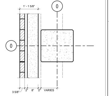
TYPICAL CAST-IN-PLACE TO PRECAST/FACE BRICK PLAN
