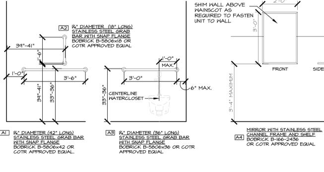
THE FOLLOWING ACCESSORIES SHALL BE PROVIDED AND INSTALLED BY CONTRACTOR ALL OTHER ACCESSORIES SHALL BE PROVIDED BY VA AND INSTALLED BY CONTRACTOR.
