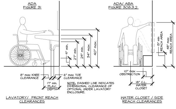
TYPICAL MOUNTING HEIGHTS FOR ACCESSORIES PROVIDED BY VA AND INSTALLED BY CONTRACTOR
