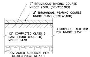
1 BITUMINOUS PAVEMENT DETAIL
