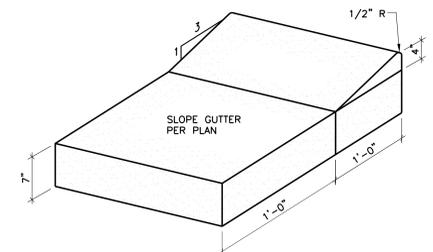
5 SURMOUNTABLE CONCRETE CURB & GUTTER (D412)
