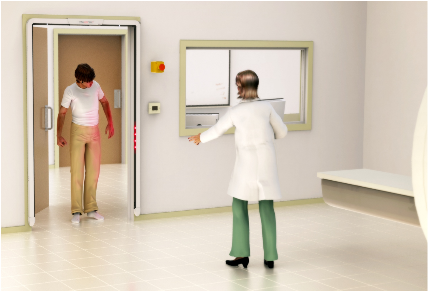
FerrAlert™ HALO II shown alarming and locating a ferromagnetic object being carried by patient about to enter the Magnet Room. Location LEDs pinpoint a potential threat.
