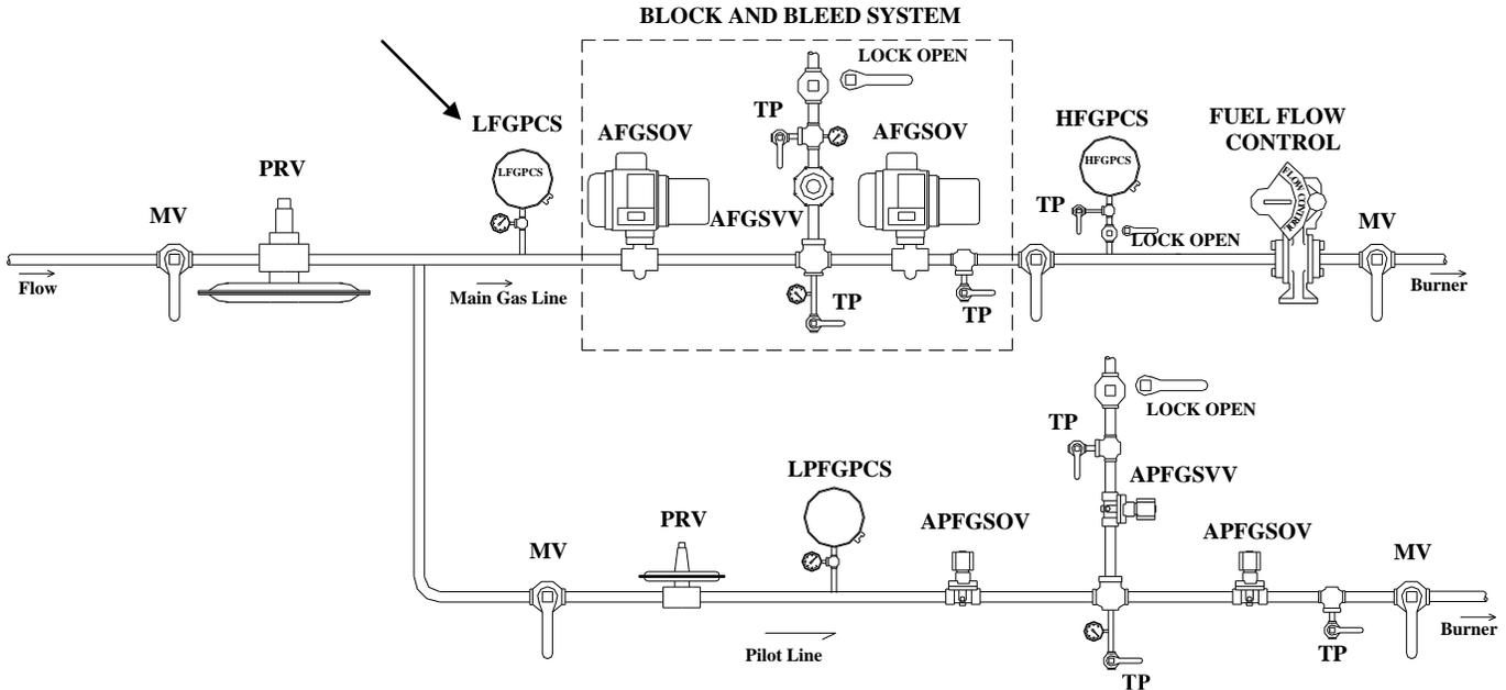
In low fire, throttle upstream fuel valve slowly until switch trips the boiler offline due to low fuel pressure but NO LOWER THAN 80% OF REGULATED PRESSURE
