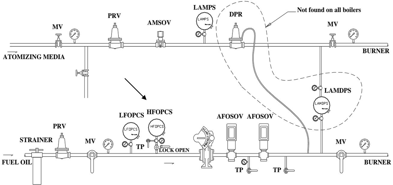
With boiler in low fire close lock open manual valve isolating the HFOPCS.
