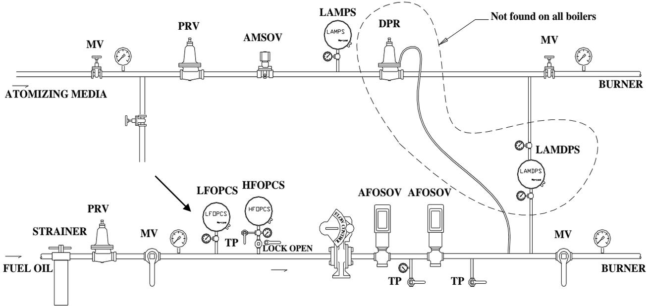
In low fire, throttle upstream fuel valve slowly until switch trips the boiler offline due to low fuel pressure but **NO LOWER THAN 80% OF REGULATED PRESSURE.**
