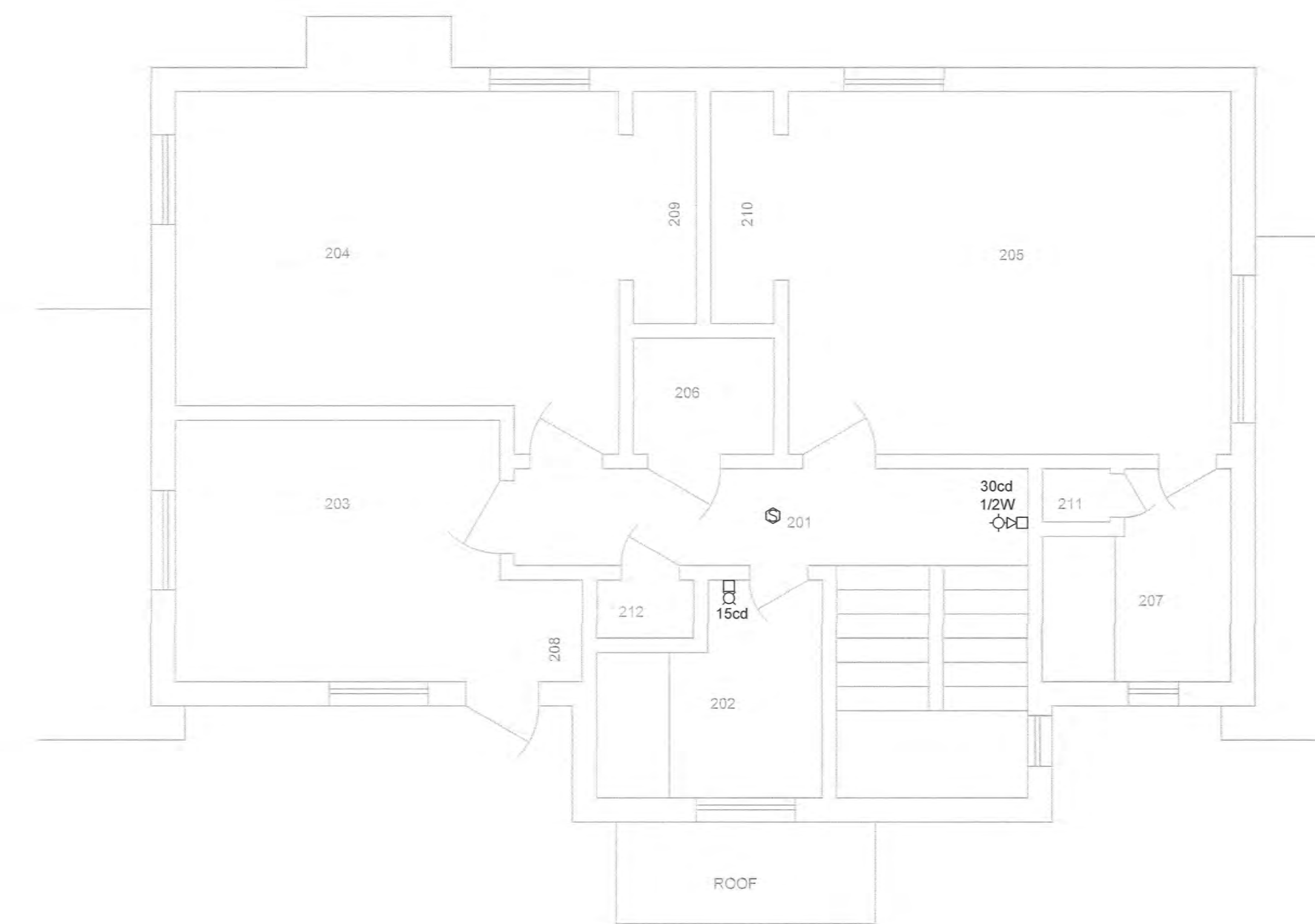
3 BUILDING 5 - SECOND FLOOR FIRE ALARM PLAN 1/4" = 1'-0"
