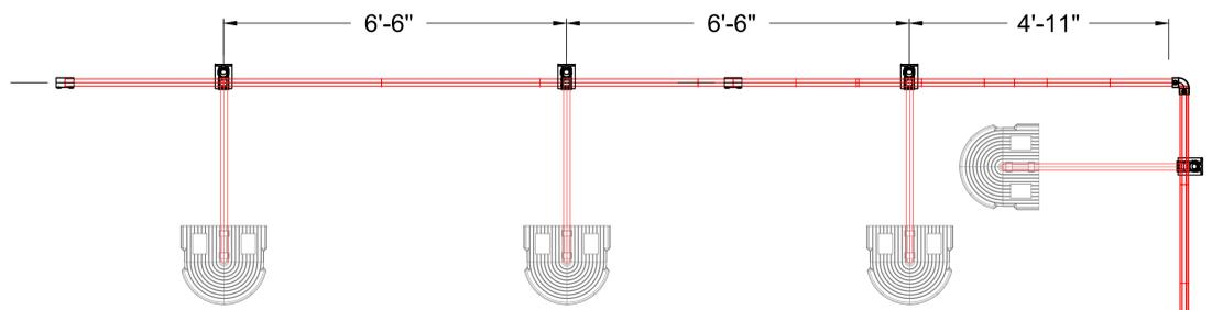
TYP. PLAN VIEW OF NON-PENETRATING ROOF RAILING (NTS)
