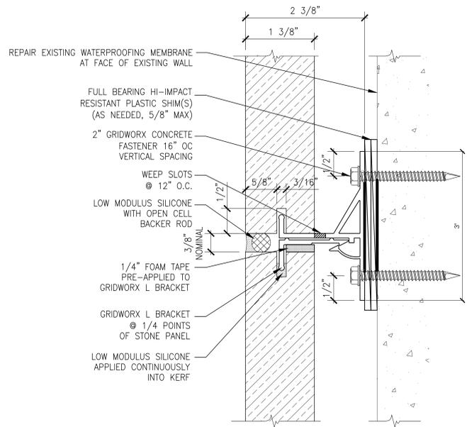
**INTERMEDIATE "T" ANCHOR SECTION DETAIL**
