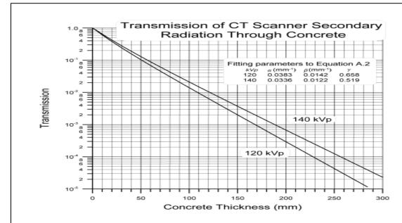
Fig. A.3. Transmission through concrete of secondary radiation from CT scanners [data of Simpkin (1991) fitted to Equation A.2].
