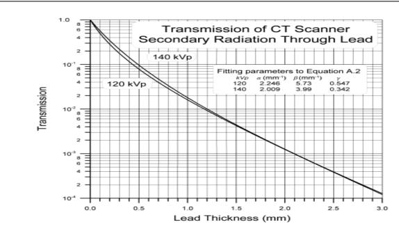
Fig. A.2. Transmission through lead of secondary radiation from CT scanners [data of Simpkin (1991) fitted to Equation A.2].
