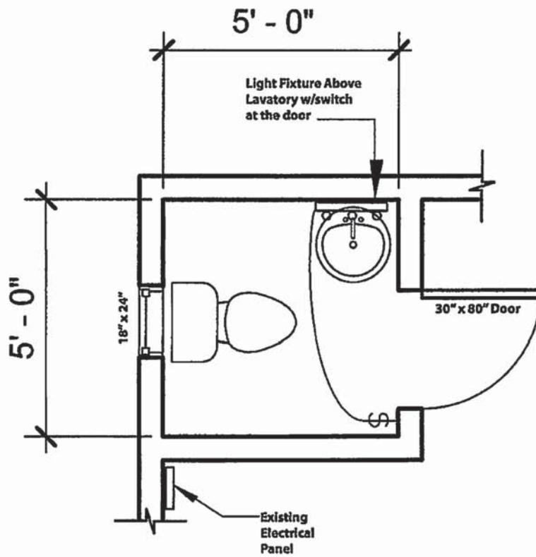
**Figure A : Schematic of 1/2 bathroom addition intended outcome**
