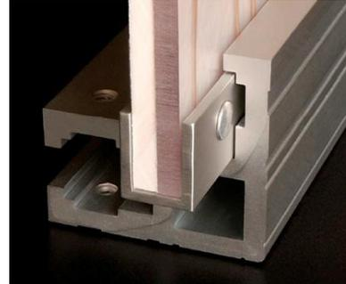
Shows channel and panel slide into corner leg, and is fastened with two set screws
