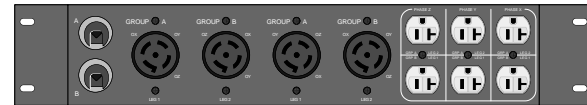
30 Amp 3-Phase PDU BASE UNIT - REAR FOUR (4) L21-20R SIX (6) NEMA 5-15/20 T-SLOT (OR EQUIVALENT)
