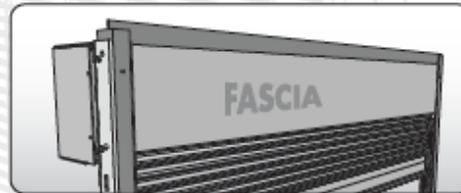
Optional hood to cover top, front and bottom of coil assembly. Optional fascia attaches to hood to cover back of coil assembly. Available in 26 Ga. steel, or 23 Ga. aluminum. (If Back of plate to Back of plate measurement is more than 10'0", a multiple piece hood is required.)
