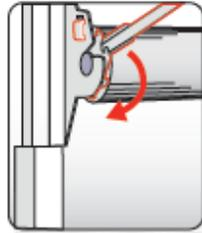
Lift Ready's attached charging arm makes wind-ing the spring easy and safe.
