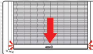
Lift Ready's exclusive Smart-Lock System allows end-users to engage the lock at a convenient height and then close the grille to the floor where the grille locks automatically.
