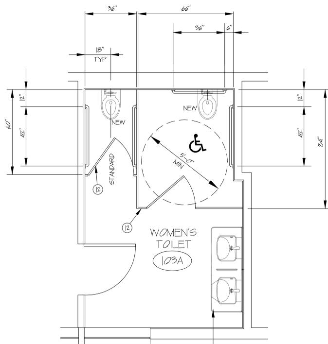
PROVIDE & INSTALL NEW LAVS. REUSE EXISTING PLUMBING, SUPPLY AND WASTE. CAP OFF UNUSED PIPING BELOW THE FLOOR & PATCH WALLS TO MATCH EXISTING ADJACENT. TYPICAL.
