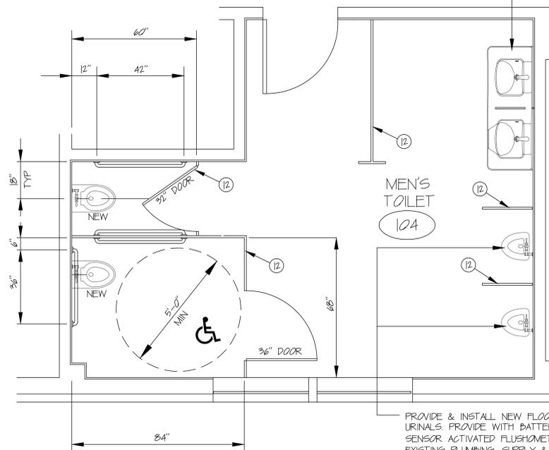
PROVIDE & INSTALL NEW FLOOR MOUNTED URINALS. PROVIDE WITH BATTERY POWERED SENSOR ACTIVATED FLUSHMETER. REUSE EXISTING PLUMBING, SUPPLY & WASTE LINES. CAP UNUSED PIPING BELOW FLOOR AND PATCH WALLS TO MATCH EXISTING ADJACENT. TYPICAL.
