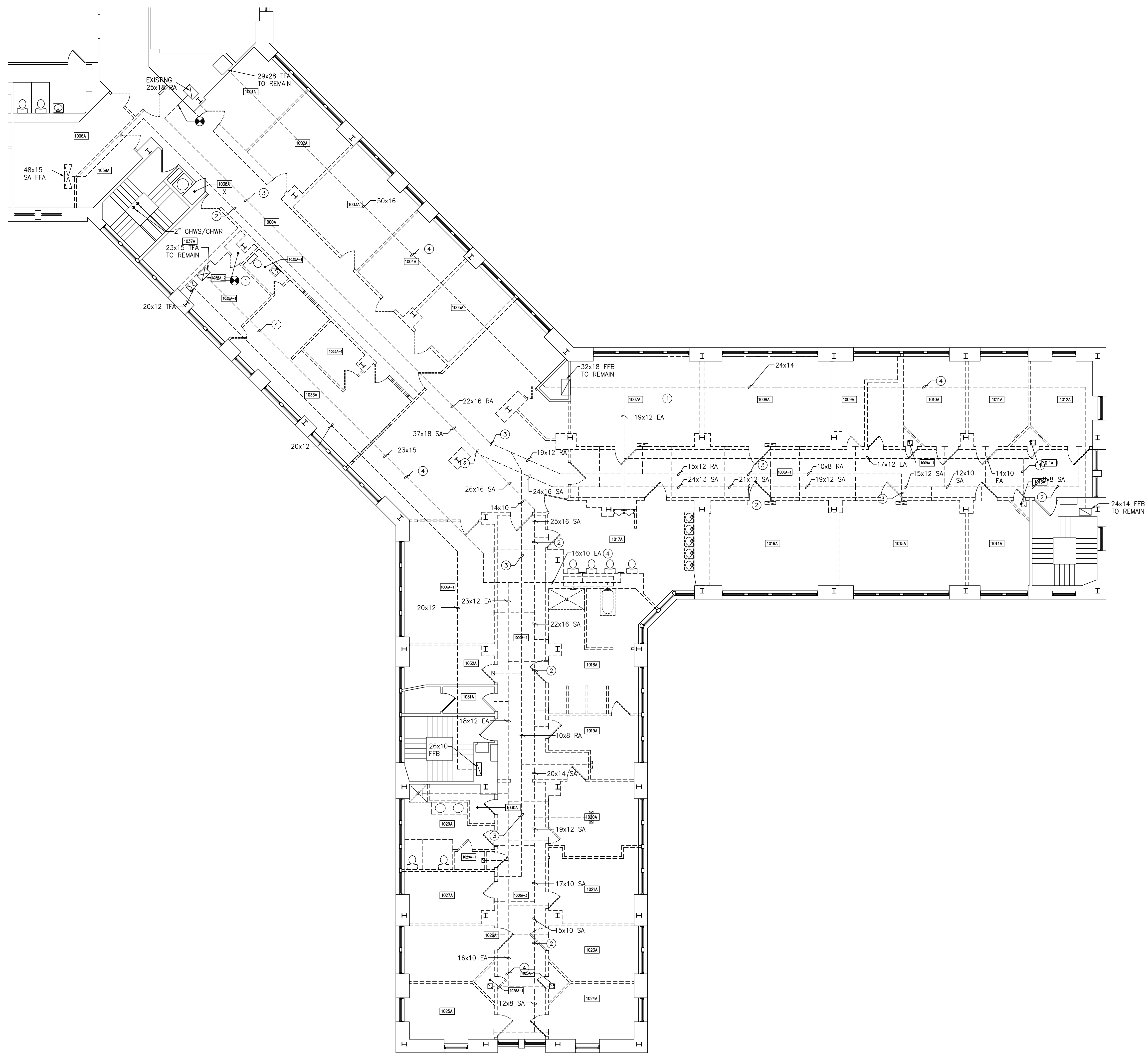
10TH FLOOR HVAC DEMOLITION PLAN 'A' WING SCALE: 1/8" = 1'
