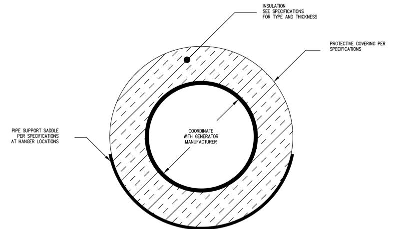
**3 EXHAUST INSULATION DETAIL**
