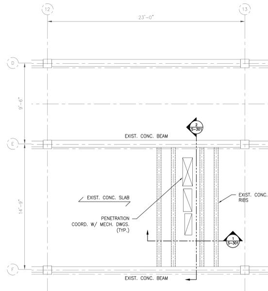
4 ATTIC - ENLARGED PARTIAL DEMOLITION PLAN
