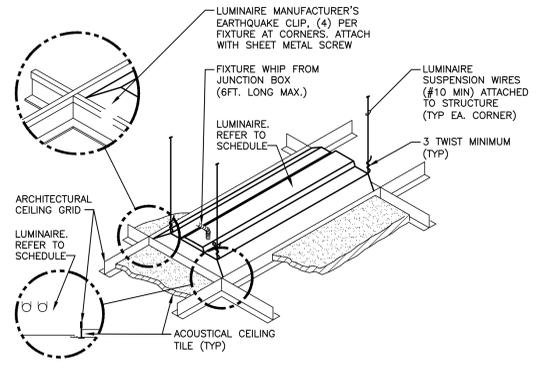
**6 LUMINAIRE MOUNTING - LAY-IN CEILING**
