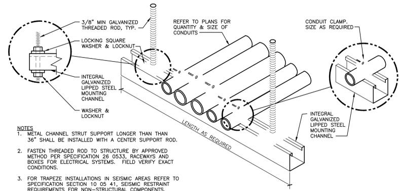
**8 CONDUIT TRAPEZE MOUNTING DETAIL**
