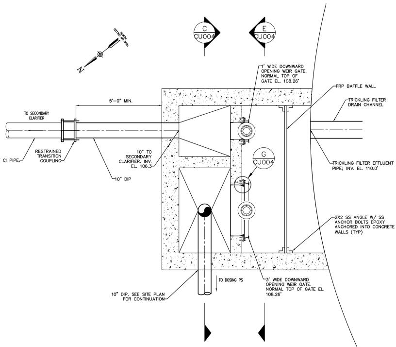
**TRICKLING FILTER SPLITTER BOX PLAN** (D) CU004
