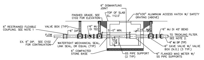
**SECTION THRU MAG METER VAULT** (B) CU004
