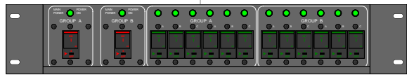
30 Amp 3-Phase PDU BASE UNIT - FRONT (ZONIT ZON-C-ZPDU1) REQUIRES TWO 30 AMP 3-PHASE (WYE) CIRCUITS WITH L21-30R RECEPTACLES (OR EQUIVALENT)
