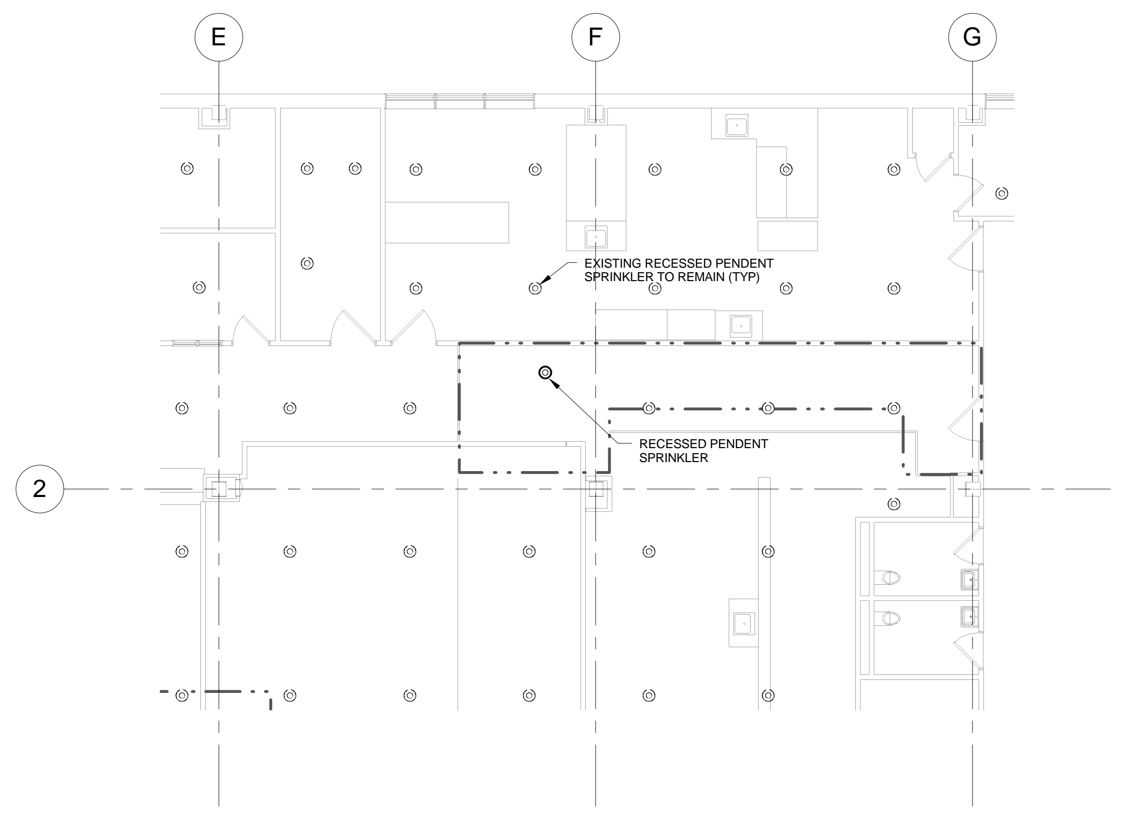
2 THIRD FLOOR PLAN - PHASE 0 FIRE PROTECTION NEW WORK SCALE: 1/8" = 1'-0"
