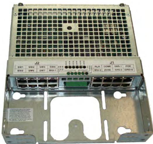
Figure 2: RCB without Cover, with Circuit Board Enclosure
