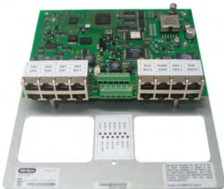
Figure 1: RCB without Cover, without Circuit Board Enclosure
