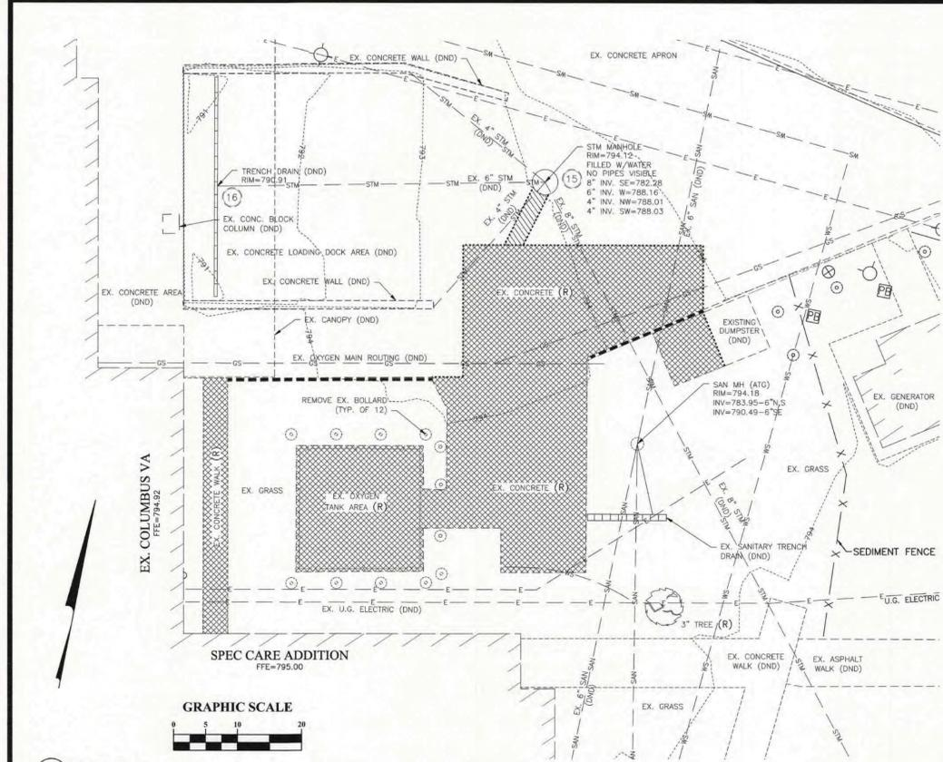
**A** DETAIL DEMOLITION PLAN
