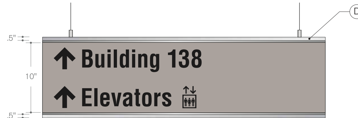
Type IN-15.52a Custom Fusion Overhead 40"w X 11.5"h Double sided suspended .080 NG acrylic lens printed second surface *no paper insert*
