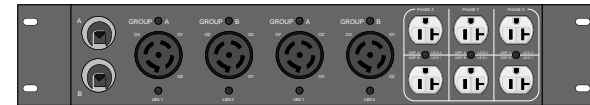
30 Amp 3-Phase PDU BASE UNIT - REAR FOUR (4) L21-20R SIX (6) NEMA 5-15/20 T-SLOT (OR EQUIVALENT)
