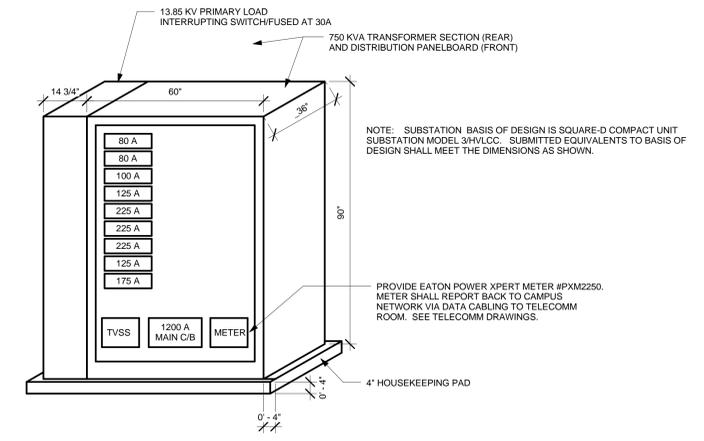
1 UNIT SUBSTATION ELEVATION
