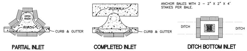
**B7 PROTECTION AROUND INLETS OR SMALLER STRUCTURES**
