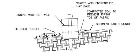
**E8 DETAIL OF PROPERLY INSTALLED HAY BALE**
