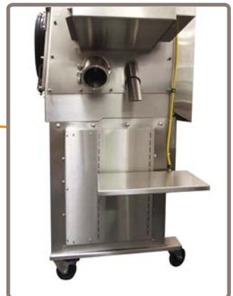
Ergonomic Placement of Sharps and Waste Tubes with Adjustable Shelf to Accommodate Different Sized Sharps Containers
