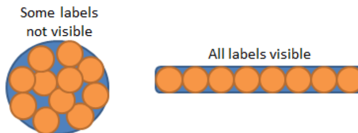
Figure 22: Cable Labels in Bundles
