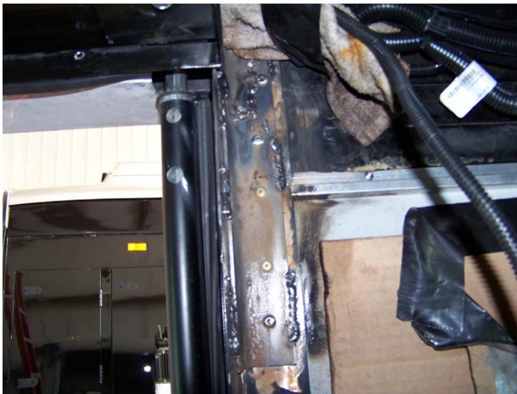
DOOR FRAMEWORK REPAIRS (5,724 TEST MILES)
