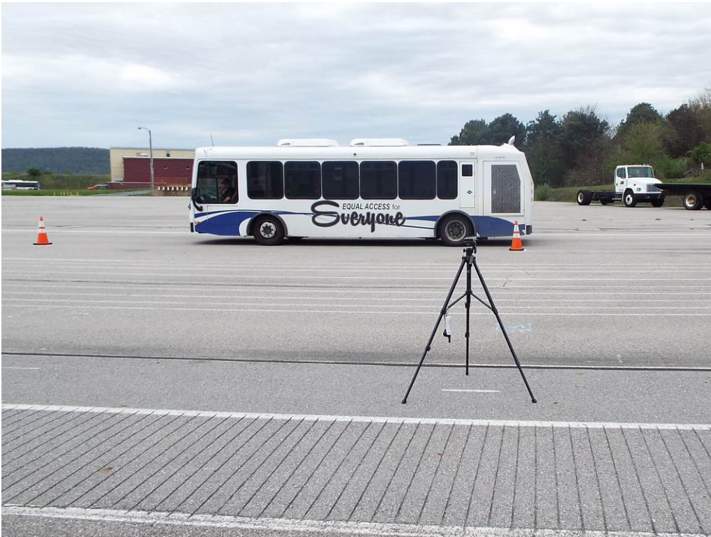
TEST BUS UNDERGOING EXTERIOR NOISE TESTING
