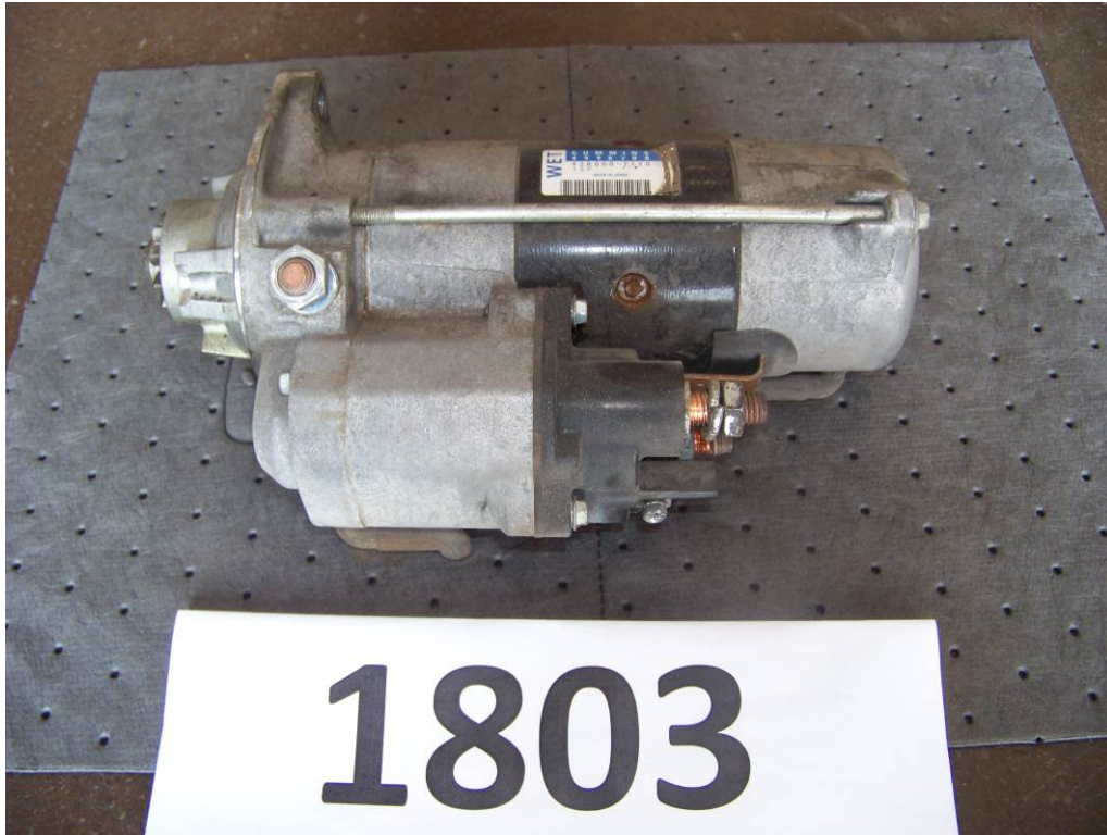
STARTER REMOVAL AND REPLACEMENT (0.3 LABOR HOURS)
