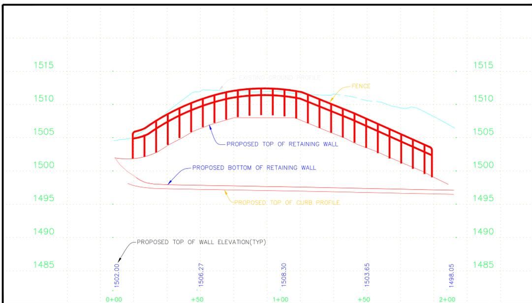
NOTE: FENCE TO BEGIN WHERE DIFFERENCE IN ELEVATION BETWEEN TOP AND BOTTOM OF WALL EXCEEDS 2'.
