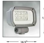
**HOUSING:** DIE CAST ALUMINUM HOUSING, DIE CAST ALUMINUM KNUCKLE. MOUNTING HARDWARE TO ATTACH TO EXISTING WOOD POLE. EXTRUDED GASKET TO SEAL LENS TO HOUSING. PROVIDE CUTOFF HOOD TO LIMIT UPLIGHT. COORDINATE FINAL AIMING WITH CONTR.
