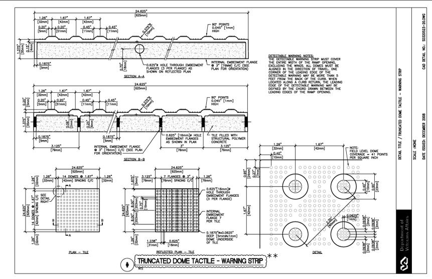
**\*\*NOTE:** CONTRACTOR SHALL USE PRECAST DOME PAVERS 2'x2'x2"; BRICK RED IN COLOR; TO MATCH PAVERS ALREADY IN USE AROUND CAMPUS.
