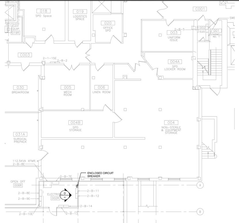
**B** ELECTRICAL PARTIAL BASEMENT FLOOR PLAN
