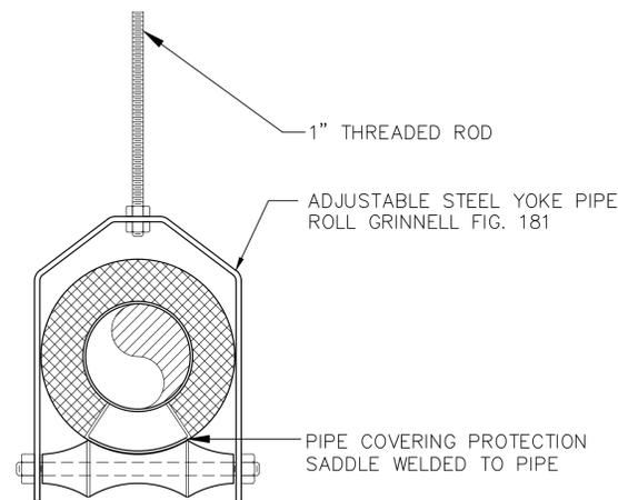
**1 HOT WATER PIPING SUPPORT HANGER DETAIL**
