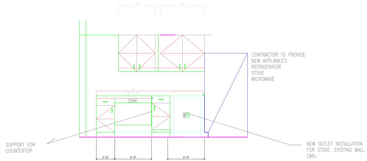
COORDINATE WITH COR FOR EXACT LOCATIONS OF NEW KITCHEN SINK, STOVE, AND STAINLESS STEEL REFRIGERATOR PROVIDED AND INSTALLED BY THE CONTRACTOR. ALL ITEMS ARE TO BE AS PER VA DESIGN GUIDE AND SUBMITTED TO THE GOV'T. FOR APPROVAL.
