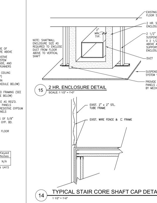
14 TYPICAL STAIR CORE SHAFT CAP DETAIL
