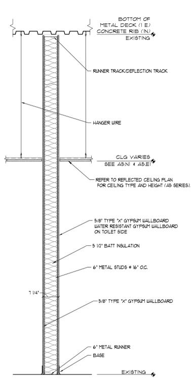
**K** K-WALL W/ GYP BOARD TWO SIDES UP TO DECK
