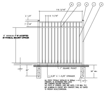
NOTE: PROVIDE APPROXIMATELY NEW FENCE IN LOCATIONS INDICATED. COMMERCIAL GRADE ORNAMENTAL ALUMINUM, STRAIGHT TOP, 10' HIGH FENCE, INCLUDING 20' ROLLING & 8' SWING GATES.
